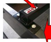
This is the sort of thing you can get done at <u>any</u> welding, engineering or fabrication shop in your own area. Simply give these instructions and photos to them. ALL holes are drilled to ½" or 12.5mm. ALL bolts are M12 Zinc Plated... @ 25mm long to attach "frame" to trailer "lip" as per and @ 65mm long to attach Trailer Racks to the "frame" as per
