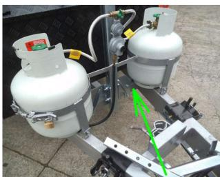
3/ Once the "new" chassis rail is welded in, paint the weld areas with "cold gal" and a "bright silver" top coat. This is a perfect match for a galvanized chassis.
