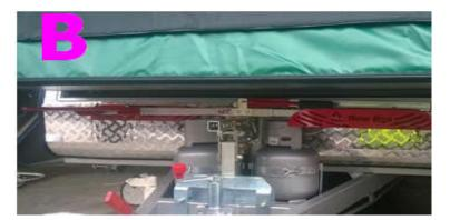
Our bolt-on mount comprises a base unit (red arrow) which fits down over an existing chassis rail on your van and a vertical post (yellow arrow).
