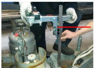
**4/** The main vertical post is a piece of 50x50x4 SHS (Square Hollow Section) tubing.
