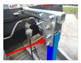
7/ Make & fit <u>at least</u> one angled brace (per red arrows) going from as high as possible on vertical post down to caravan chassis.
